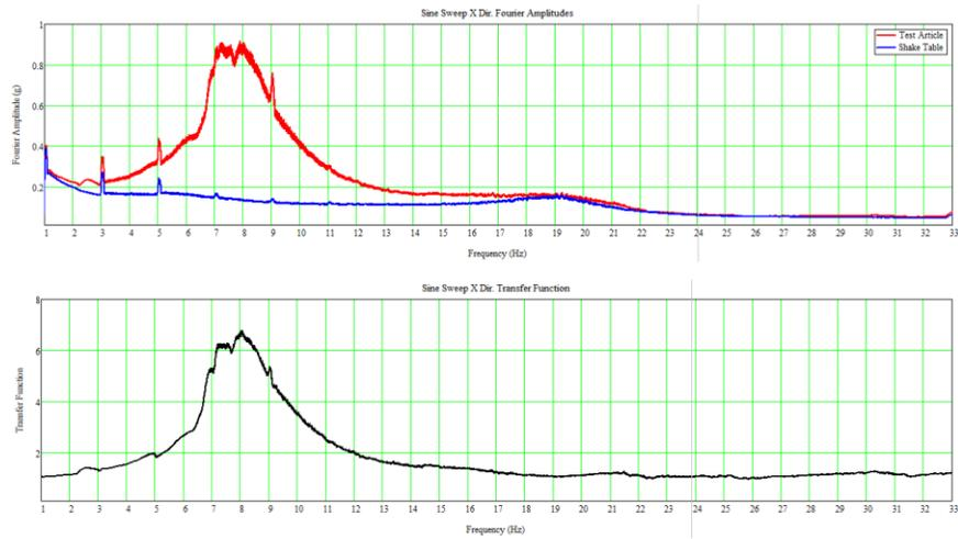
Figure 9. Fourier Amplitudes and Transmissibility Function for Test Article in the X Direction.
