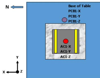
Figure 4. Instrumentations layout.
