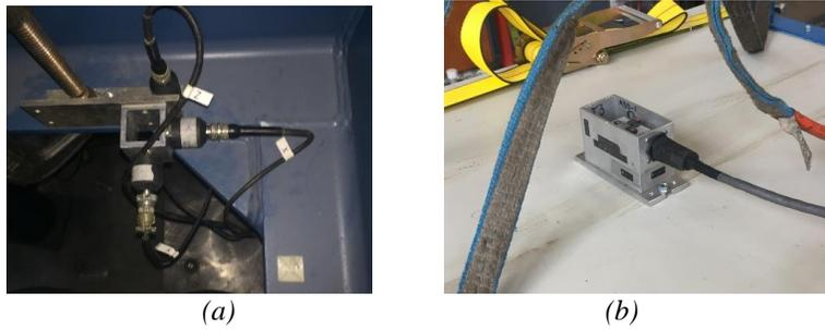
Figure 5. Instrumentations used in testing program: a) PCBI Sensors; b) ACI Sensors.
