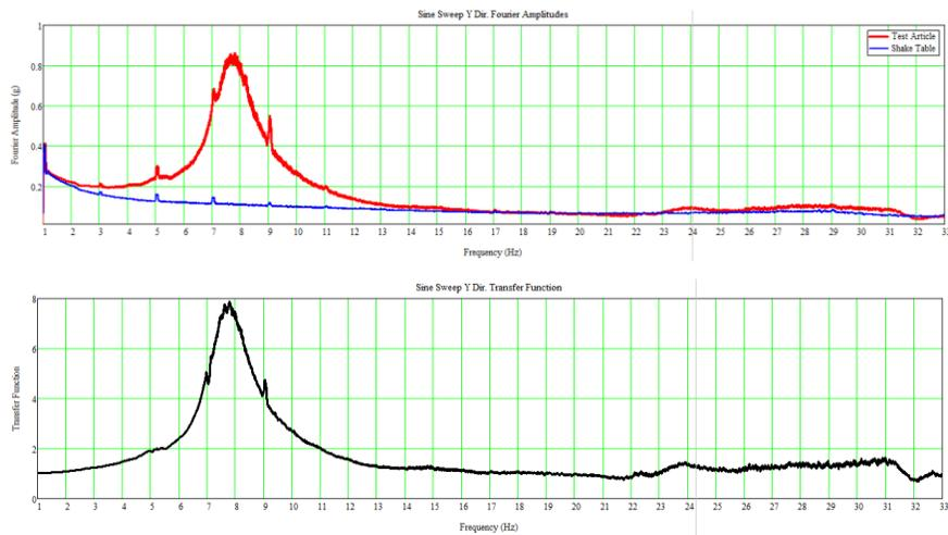
Figure 10. Fourier Amplitudes and Transmissibility Function for Test Article in the Y Direction.
