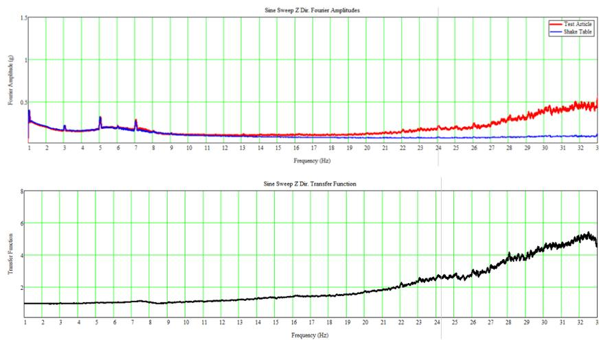
Figure 11. Fourier Amplitudes and Transmissibility Function for Test Article in the Z Direction.
