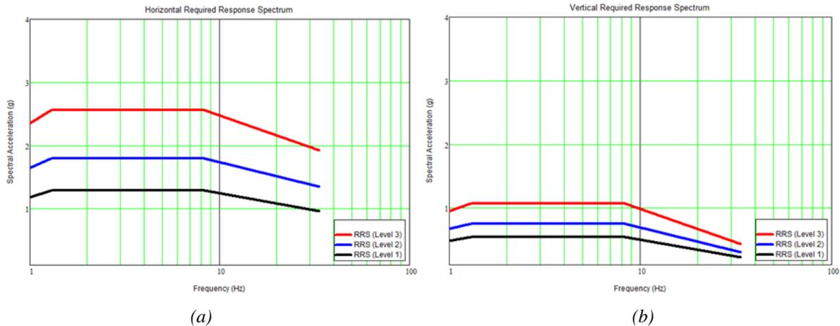
Figure 8. AC 156 Required Response Spectrum (RRS) for time history tests, 5% Damping: a) Horizontal; b) Vertical.
