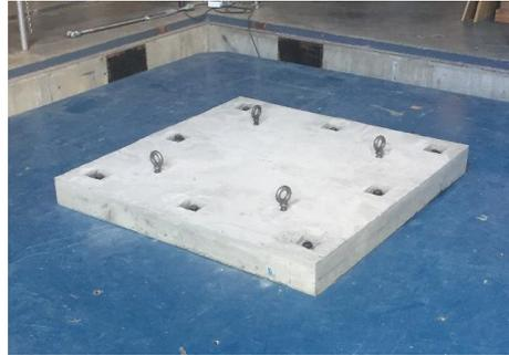
Figure 2. Concrete slab installed on the Shake Table.
