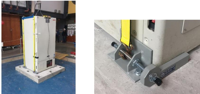
Figure 3. Test setup and EQ Restraint System (EQRT 203-7) installed on the equipment prior to testing.
