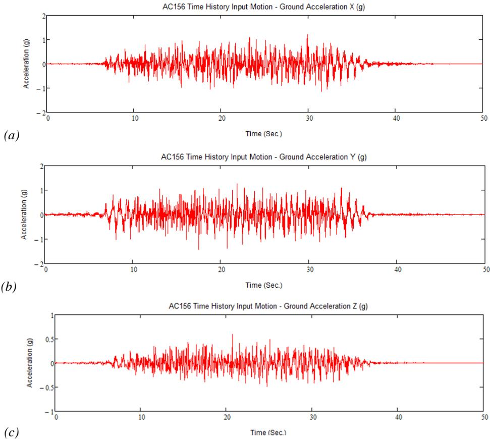
Figure 6. AC 156-time history motion records used for Shake Table tests: a) Horizontal X direction; b) Horizontal Y direction; c) Vertical Z direction.
